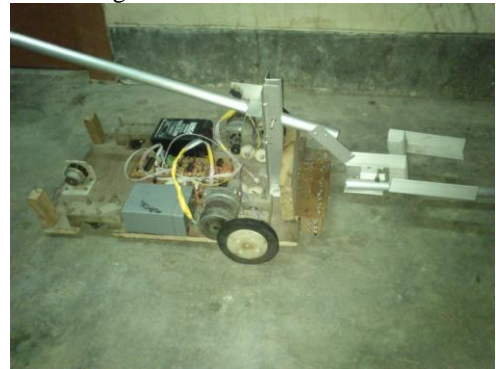
Fig.5 Complete picture of the robot with mechanical gripper
